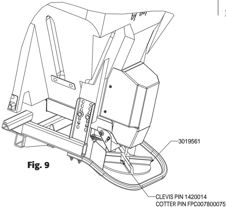
10. Install lid #3015926 on to hopper. Place lid on hopper. Bend hinges outward from center of the hopper. Slide hinges openings on round protrusions of the lid. Repeat this operation on opposite side of the hopper. Secure lid on hopper using lynch pin. To open lid from either side of the hopper disengage lynch pin, bend both hinges outwards and open lid.
