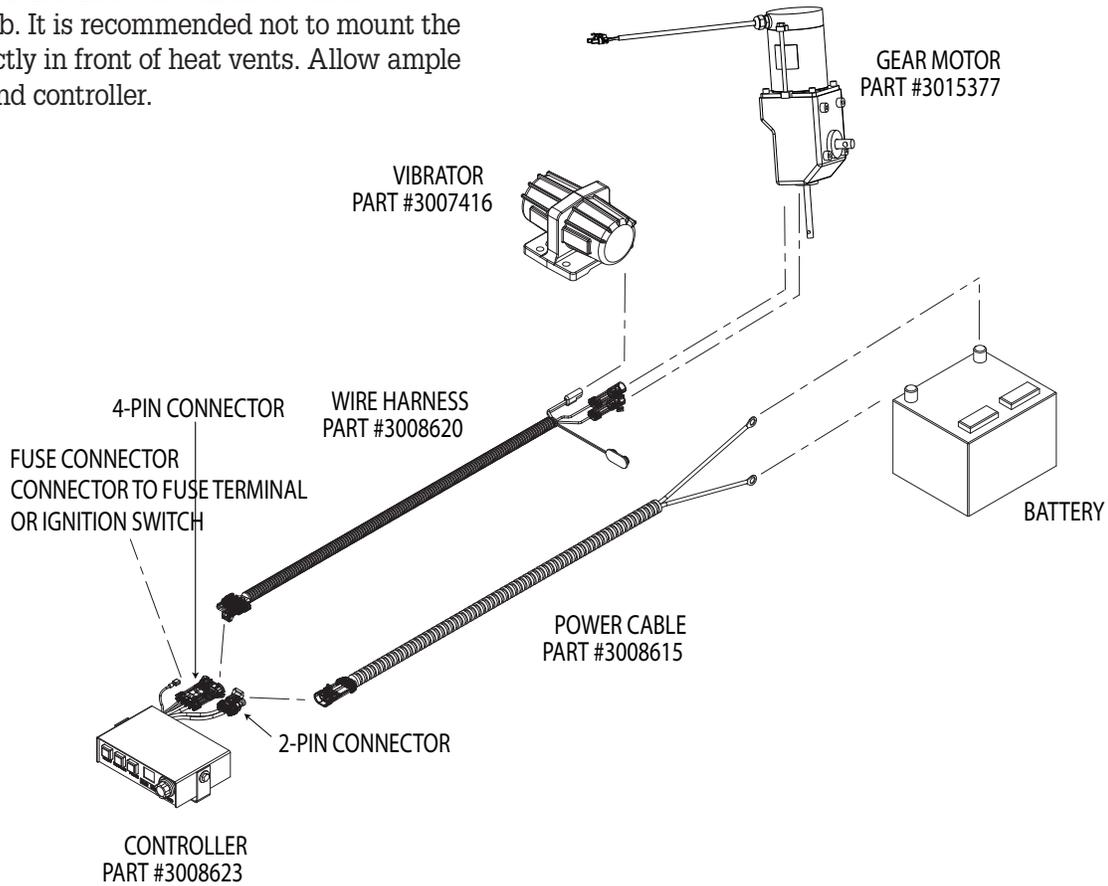
**Installing Controller and Wiring**
