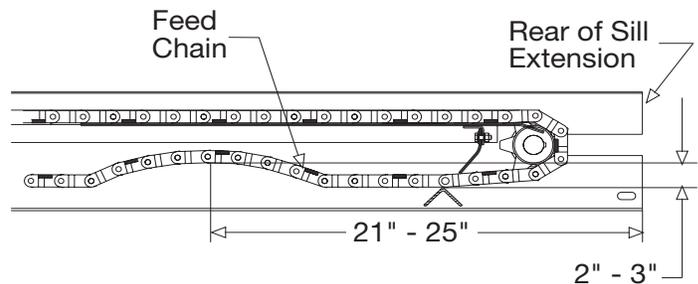
To check the tension, measure in 21"-25" from the rear edge of the gear box mount. Push up on the chain with your hand. The conveyor chain should lift up 2"-3" off the conveyor chain guide or cross angles.
