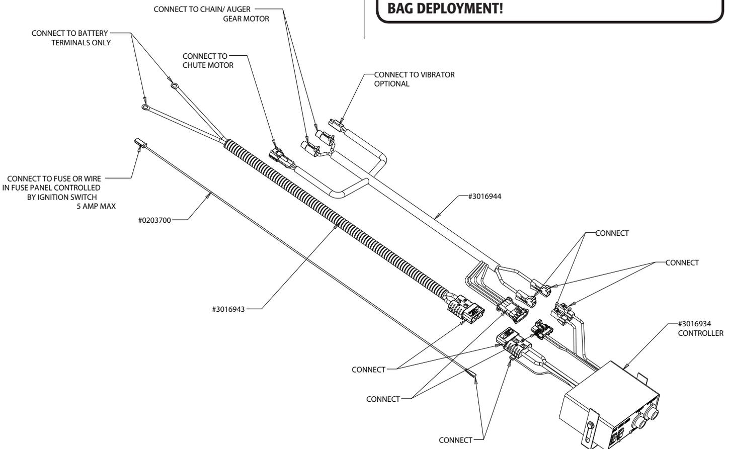
**B.** Route both wire harnesses into truck cab through firewall (it maybe necessary to drill holes). Insulate hole to avoid water leaks.
