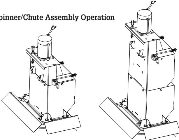
Attach chute to hopper assembly by inserting tabs into slots in chute motor plate. Then secure chute by engaging spring latches in respective holes. Chute heights can be adjusted by attaching lower chute weldment to the upper one using upper or lower set of holes. Two sets of holes are located on the bottom of upper chute weldment and under internal baffles selectors.
