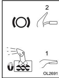
Squeeze Attachment Clutch Lever against handlebar (1) to engage attachment. Release both clutch levers (2) to disengage power and apply brake to attachment.
