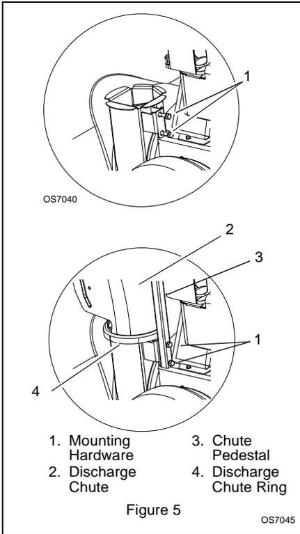
4. Remove the cover from the gear assembly on the discharge chute.
