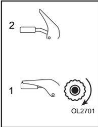
Squeeze the Traction Drive Clutch Lever against the Handlebar (1) to engage wheel drive for propelling unit. Forward speed will vary according to snow depth and moisture content.
