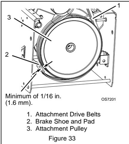
2. If there is less than 1/16 in. (1.6 mm) gap between brake pad and belts, follow these steps:
