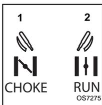
1. Choke Closed position: chokes off air to engine for easier start.
