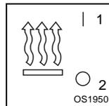
Turn the heated handles switch to the ON (1) position to activate. Turn the switch to the OFF (2) position to deactivate.
