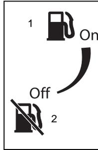
**IMPORTANT:** The fuel shut-off valve **MUST** be in the closed position prior to transporting the unit.
