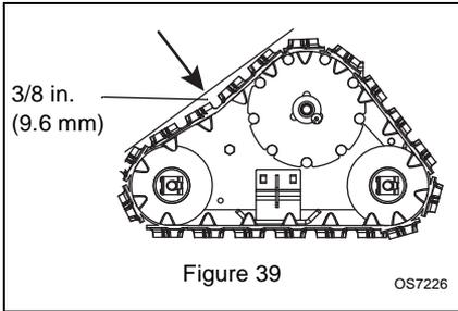
If unit pulls to the left or right when a straight path is desired adjust the track tension. If the unit is pulling to the left, tighten the left track adjuster. If the unit is pulling to the right, tighten the right track adjuster.
