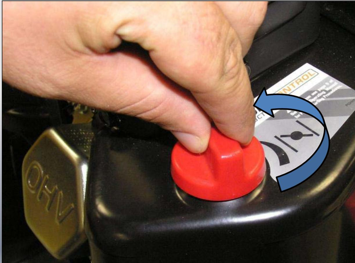
Allow the engine to warm up for approximately 30 seconds before slowly rotating Choke Knob to Run position.
