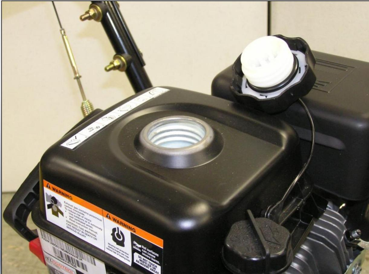
Fill fuel tank. DO NOT OVERFILL! See *FILLING FUEL TANK* in Owners Manual.
